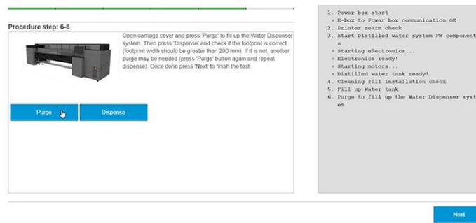
Then, tap **Dispense** and check if the water footprint is correct (the footprint width should be greater than 200 mm). If not, another **Purge** may be needed (tap the **Purge** button again and repeat **Dispense**).
