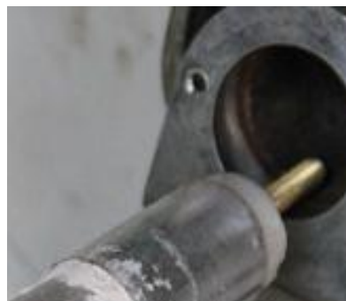
3. Put heater into upper roller.
