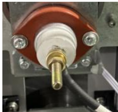
1. Install lead wire, flat mat and hex nut as pic.
