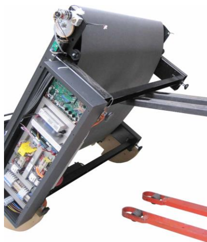
FIGURE 14 USE ONLY TOP OF THE FORKS
