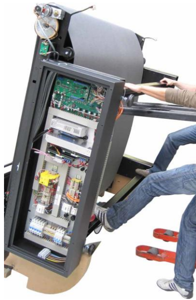
FIGURE 13 PULL TABLE BACK ON PALETTE STACKER
