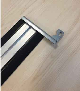
2. Remove one of the side brackets, using a T20 screwdriver.
