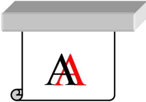
The printheads may be misaligned if you have not aligned the printheads for a long time, or if there has been a substrate jam. Align the printheads if necessary (see [Align the printheads on page 154](#)). You can check whether it is necessary by printing the printhead alignment status plot (see [Alignment status plot on page 218](#)).
