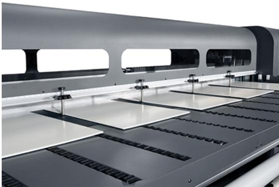
Use the built-in substrate alignment pins for quick positioning of the sheets across the printer's width. Align the left side of each sheet with one of the pins, with a small space from the right edge of the sheet to the next pin, to allow for variations in sheet dimensions. Alternatively, if you position the pins with zero clearance between the sheets and each pin, before each print be sure to raise the pins over the thickness of the sheets; otherwise the sheets could become skewed.
