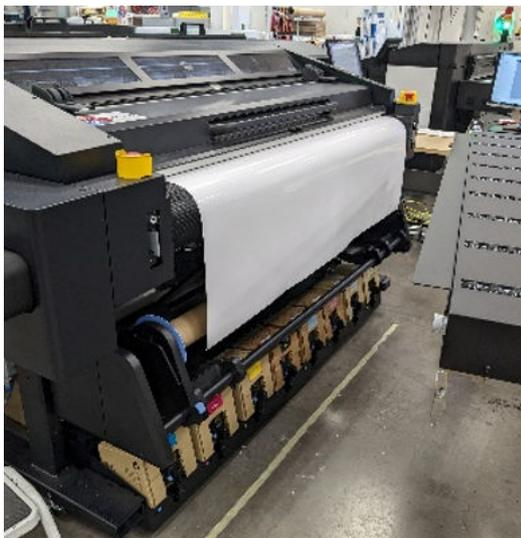
4. Pull down the center of the substrate's leading edge to straighten the substrate. Do not attempt to pull more substrate out of the printer.
