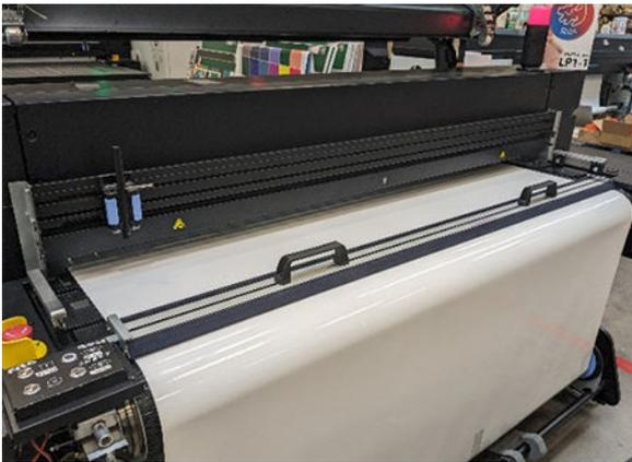
4. Ensure that the pins fit into the holes at the edges of the brackets.
