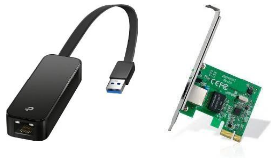
Figure 6: USB to ethernet adaptor (left) and PCIe ethernet card (right)
